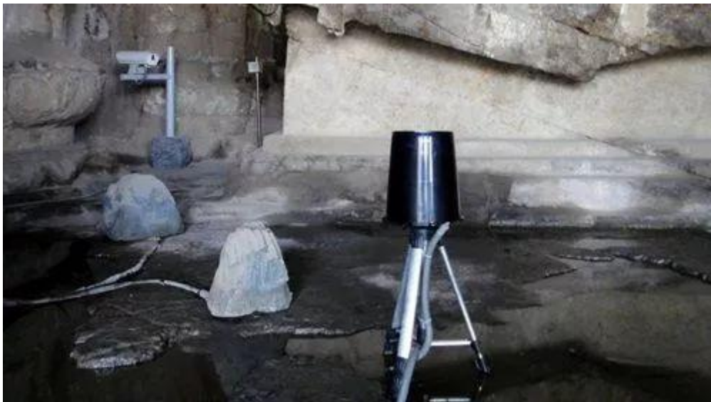
Figure 1-3-1 - Infrared Cameras and Water Seepage Monitoring Instruments in the Cave
